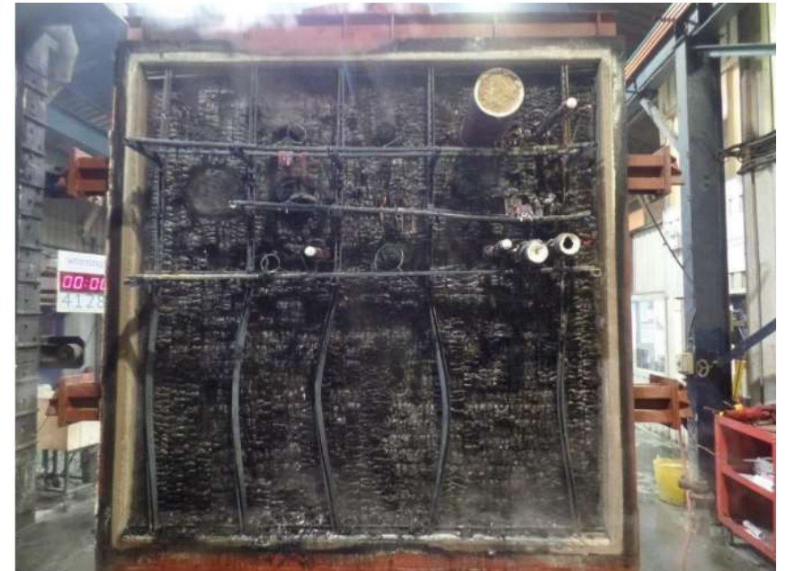
Fire exposed side of a timber construction tested with Protecta products
