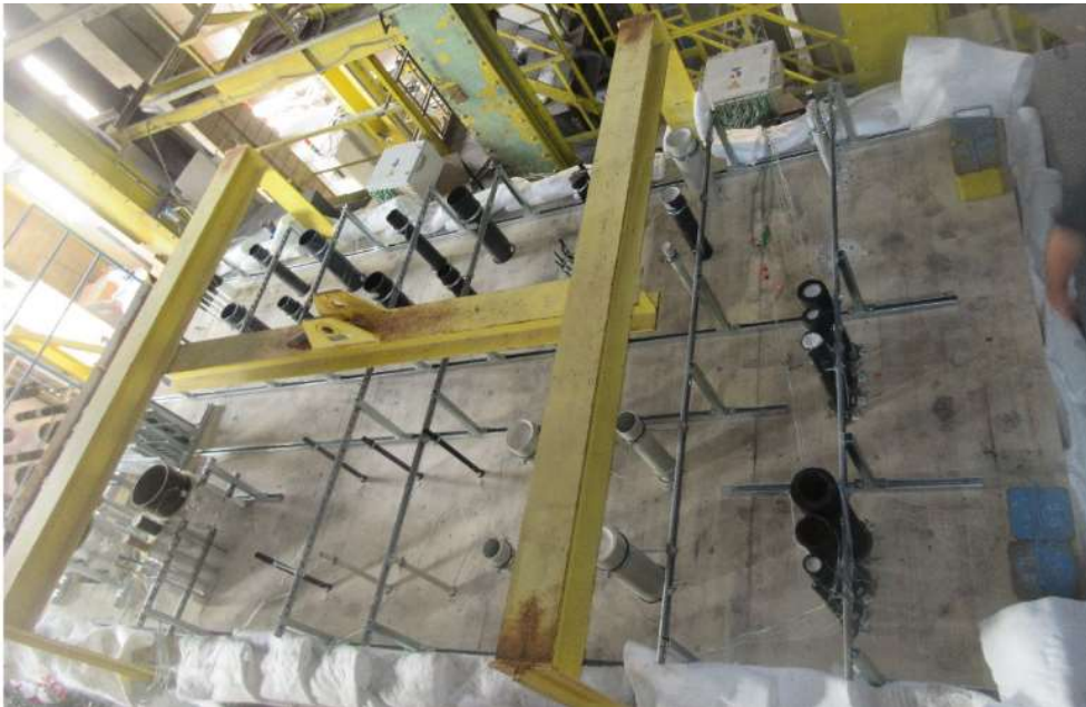
Test of a timber floor with service penetrations fire sealed with Protecta products
